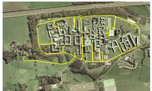
Duct route as installed
